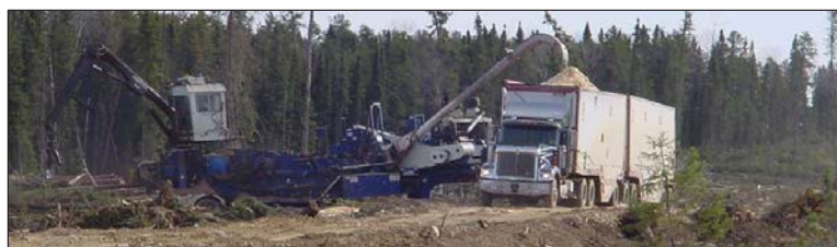
Roadside chipping operation.
