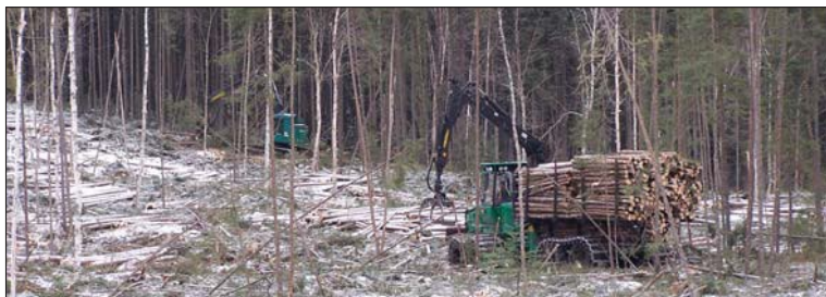
Cut to length operation.
