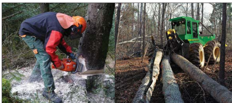
Cut and skid operation.
