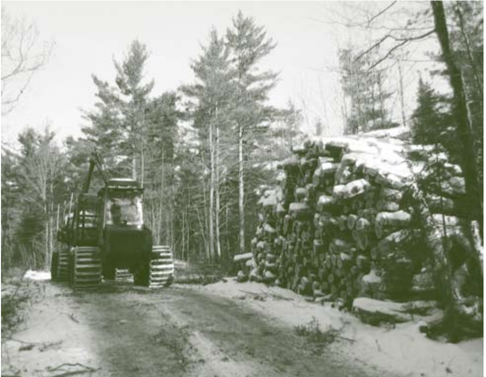
The forwarder seen in this photograph is equipped with wide tracks to provide better floatation and minimize site damage (e.g., compaction).
