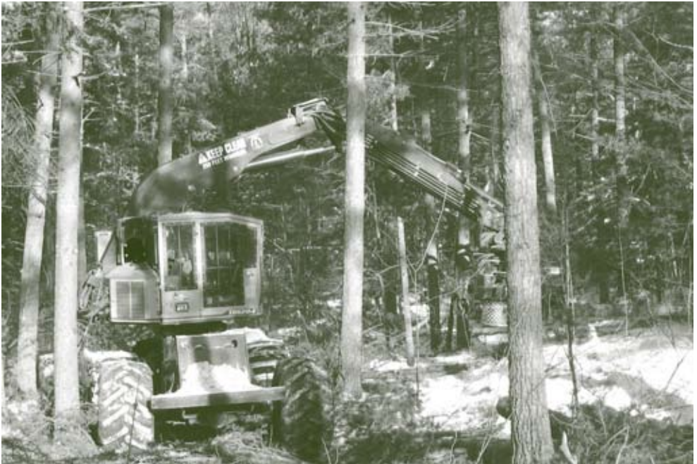
Specialized cut-to-length mechanical harvesters are often used in conifer plantation thinning operations.
